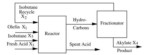
$X_1$  = Olefin feed (barrels per day)  $X_6$  = Acid strength (weight percent)  $X_2$  = Isobutane recycle (barrels per day)  $X_7$  = Motor octane number alkylate
