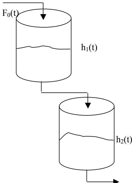
3. Consider the two tanks in the figure with levels  $h_1$  and  $h_2$  for each tank and cross sectional areas of  $A_1$  and  $A_2$ . The inlet flowrate to the first tank is  $F_0(t)$  and the outlet flows for tanks 1 and 2 are given by  $C_V (h_1)^{1/2}$  and  $C_V (h_2)^{1/2}$ , respectively.
